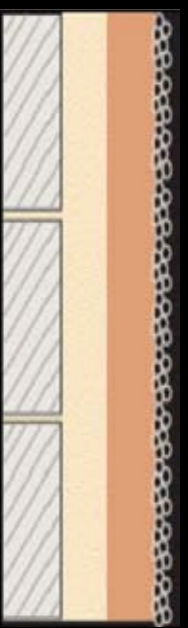
Base Coat 8-10mm Dash Receiver 8mm Dry Dash
