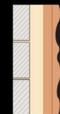
Base coat 10-12mm Dash receiver 4-6mm Roughcast
